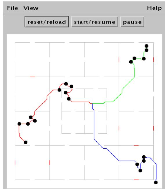
Fig. 4. PRIM ALLOCATION in TEAMBOTS (3 robots, 20 targets).
