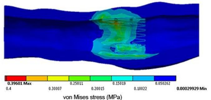
Fig. 4 Arterial wall von Mises stress results
