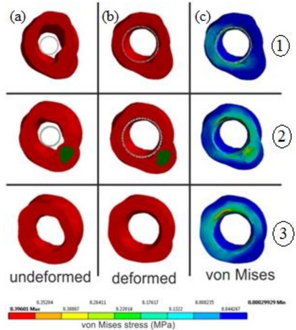
Fig. 3 (a) Undeformed arterial wall and plaque, (b) Deformed arterial wall and plaque, (c) Arterial wall and plaque Von Mises stress, for the three cross sections indicated in Fig.2
