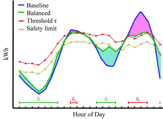
Fig. 1: Example shifting procedure. The purple-shaded load during  $t_h$  must be shifted to non peak intervals  $t_l$ .
