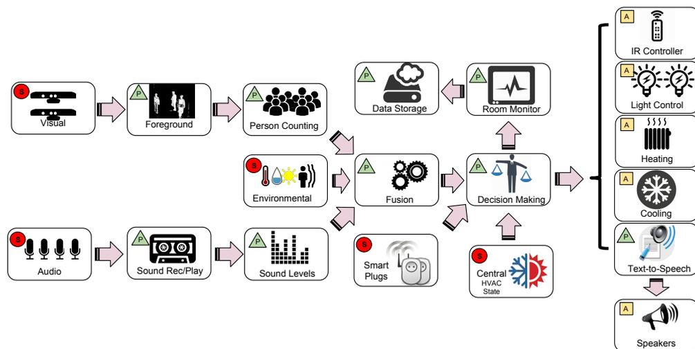
Figure 1: High-level architecture of the smart room application.
