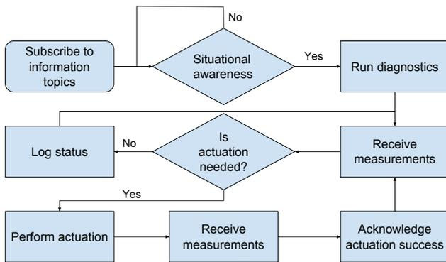
Figure 3: Flowchart of the DM's functionality.
