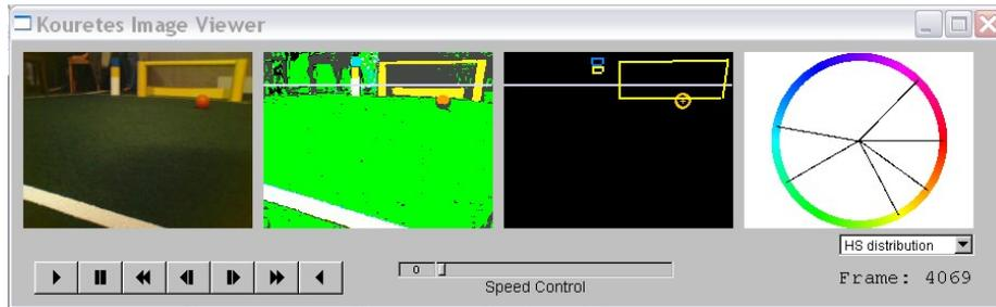
**Fig. 3.** Histogram-based visual object recognition: camera image, segmented image, recognized objects, color separation.
