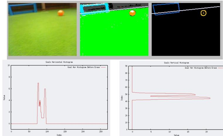
**Fig. 4.** Goal recognition: raw image, color-segmented image, recognized objects
