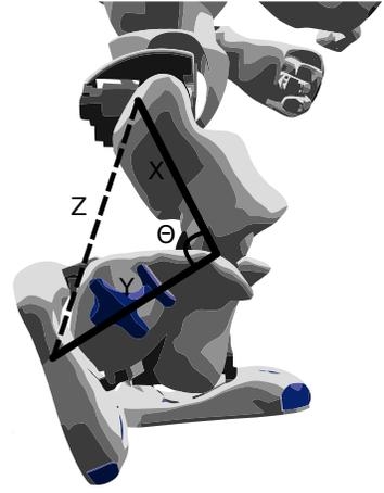
Fig. 2. Triangle formed by the robot leg
